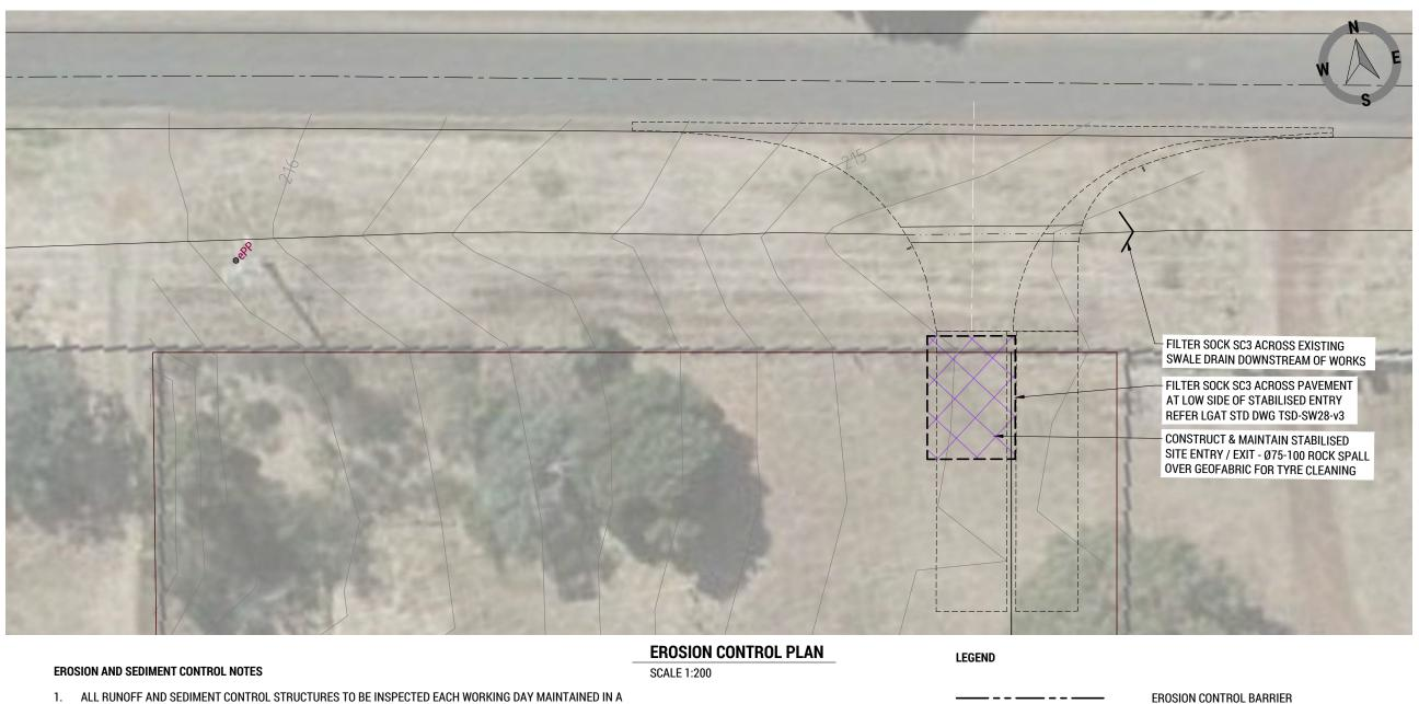
ALL RUNOFF AND SEDIMENT CONTROL STRUCTURES TO BE INSPECTED EACH WORKING DAY MAINTAINED IN A FUNCTIONING CONDITION
